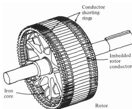
Figure 1.3. Squirrel cage rotor construction (From Ref. 9.)
