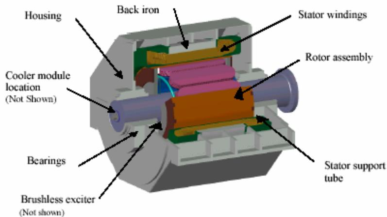
Figure 4.1. 25 MW, 120 RPM ship propulsion motor (From Ref. 23.)
