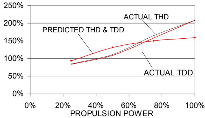
Figure 8.4. Filter current distortion (From Ref. 31.)
