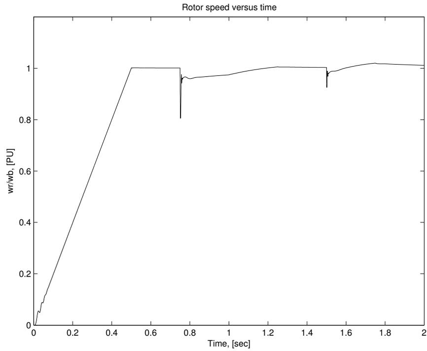
Figure 9.9. 30-MW motor speed response to load changes
