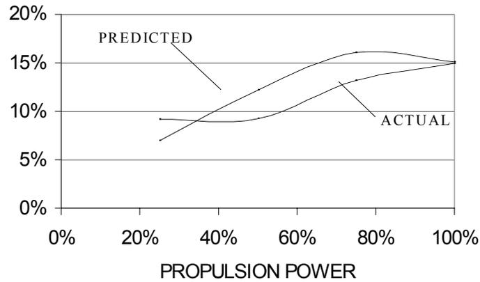
Figure 8.6. Generator voltage distortion (From Ref. 31.)
