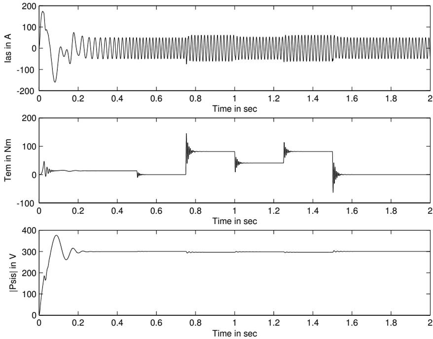
Figure 9.7. 15-kW motor simulation (From Ref. 32.)
