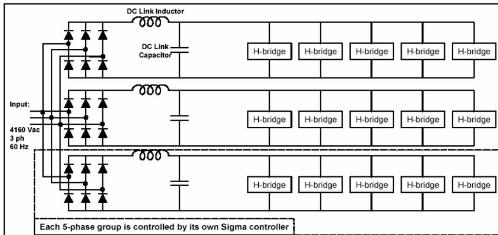
Figure 8.2. IPS PWM converter schematic (From Ref. 32.)
