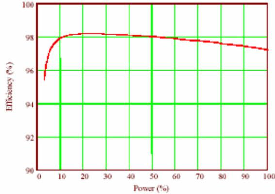
Figure 4.2. HTS motor efficiency at partial-load (From Ref. 23.)
