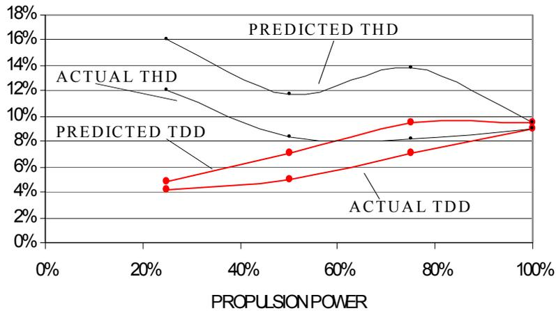
Figure 8.5. Generator current distortion (From Ref. 31.)
