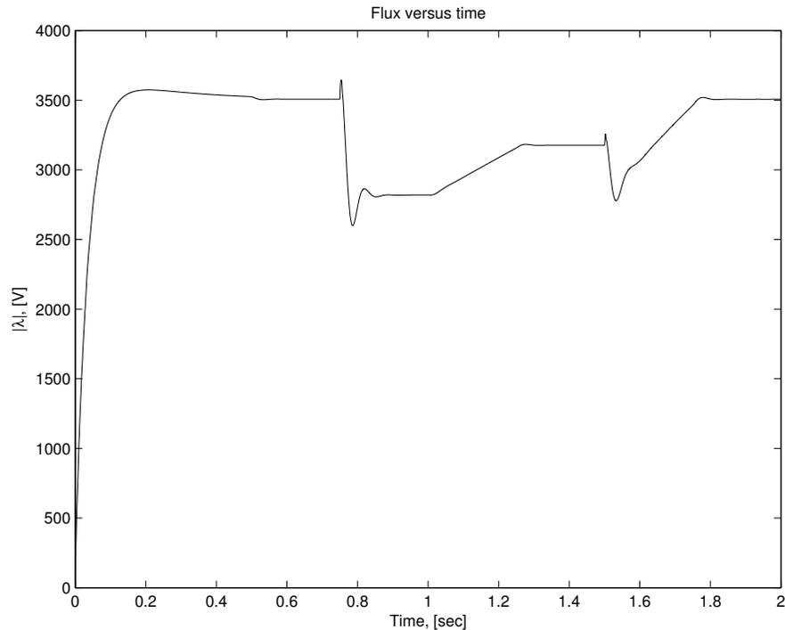
Figure 9.13. Flux response to load changes
