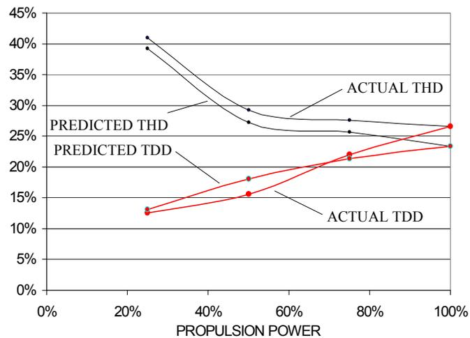
Figure 8.3. Converter current distortion (From Ref. 31.)
